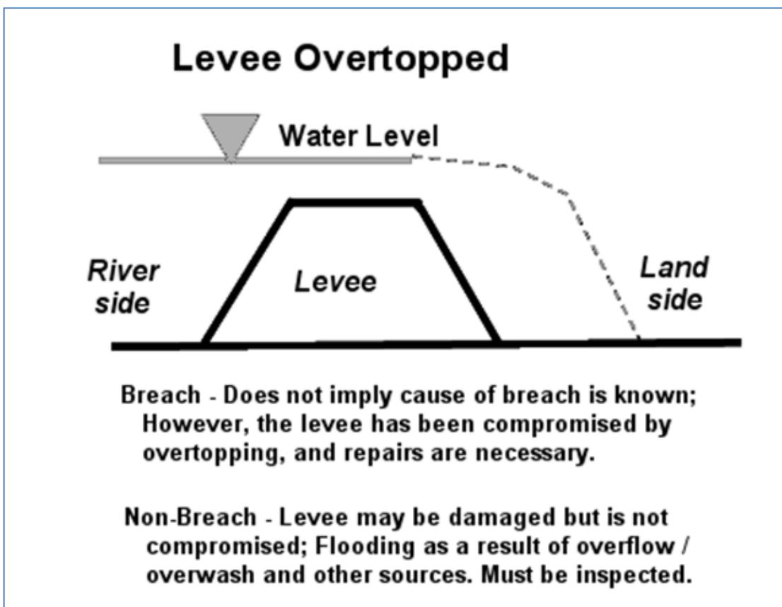
**Figure 9 – Possible results when levee is overtopped.**
