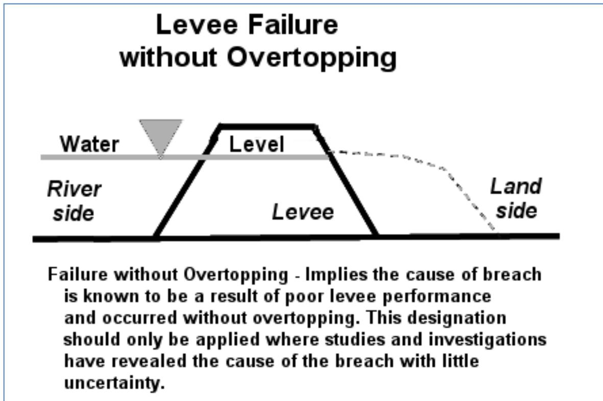
**Figure 10 – Failure Breach**
